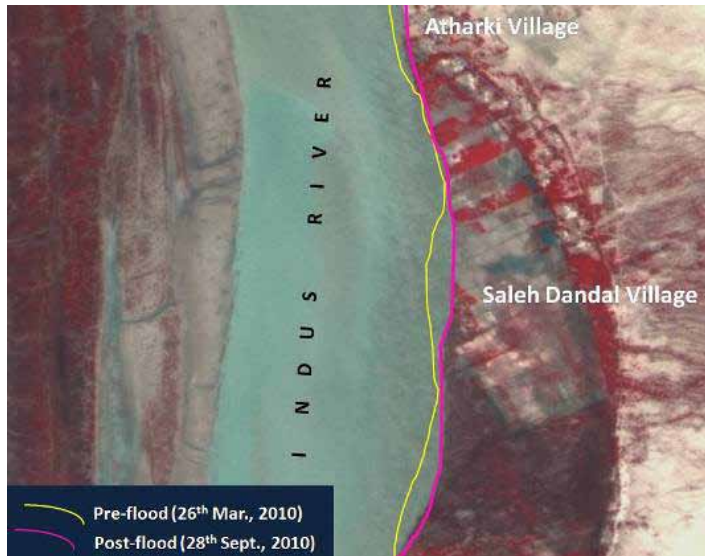
Figure 6: Land erosion status due to flood 2010
