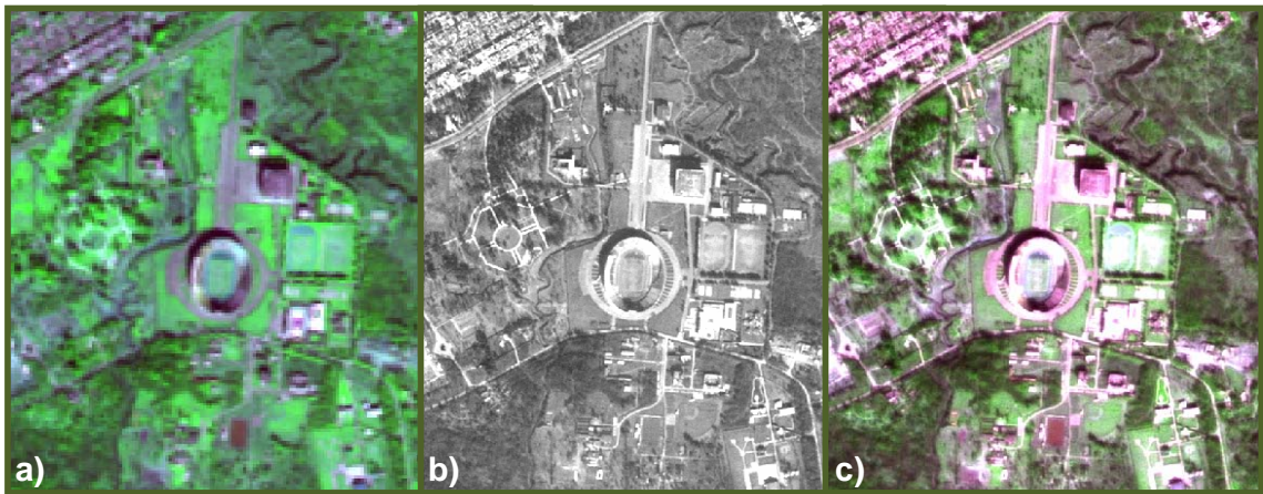
Figure 5: SPOT (a) multispectral, (b) panchromatic and (c) high resolution merged imagery
